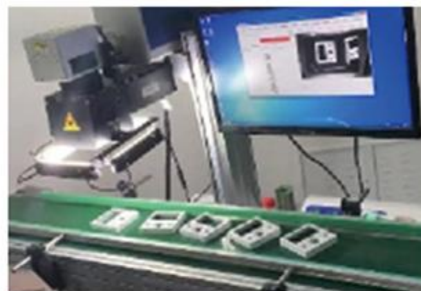
• Control panel visual laser marking
